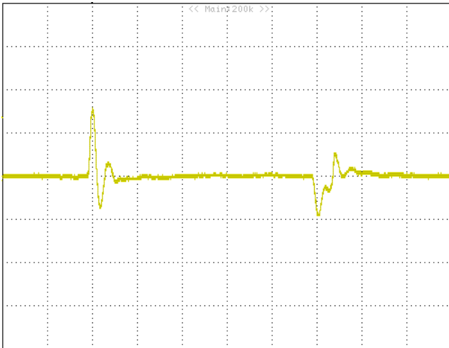
Figure 19: Transient response to dynamic load change at 2.5A/\mu S from 50%~ 100%~50% of I_o , max at 7Vin, 0.69Vout (Cout = 1uF ceramic, 47uF*2 +10uFceramic) Yellow : VOUT, 0.2V/div, 100uS/div
