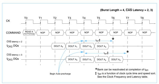
Although a Read Command with auto-precharge can not be interrupted by a command to the same bank, it can be interrupted by a Read or Write Command to a different bank. If the command is issued before auto-precharge begins then the precharge function will begin with the new command. The bank being auto-precharged may be reactivated after the delay t<sub>RP</sub>.
