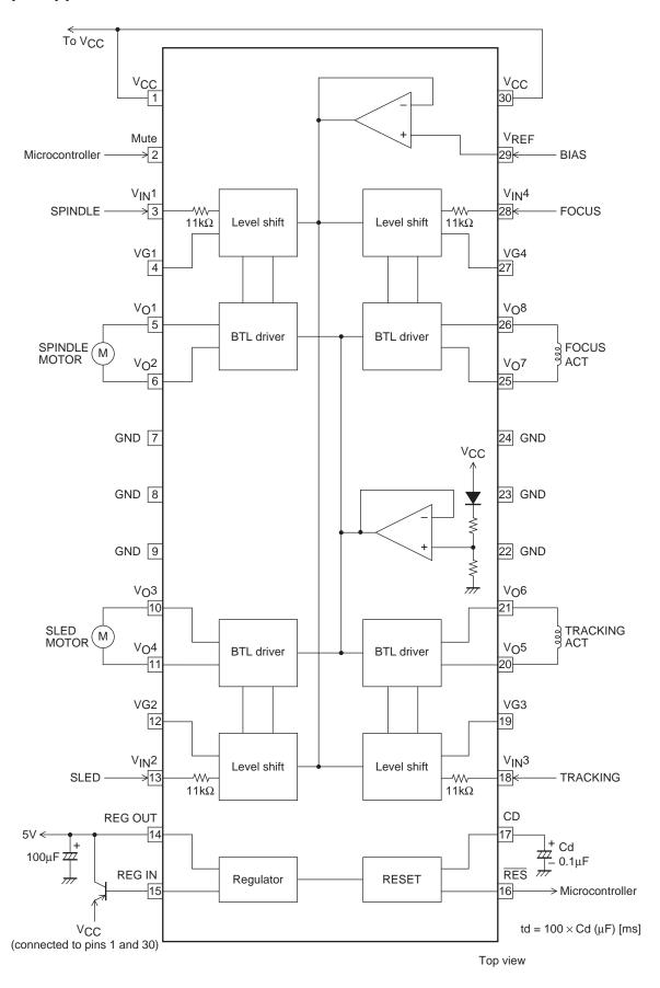
Note: Use a delay capacitor (Cd) whose capacitance does not change much according to the temperature.
