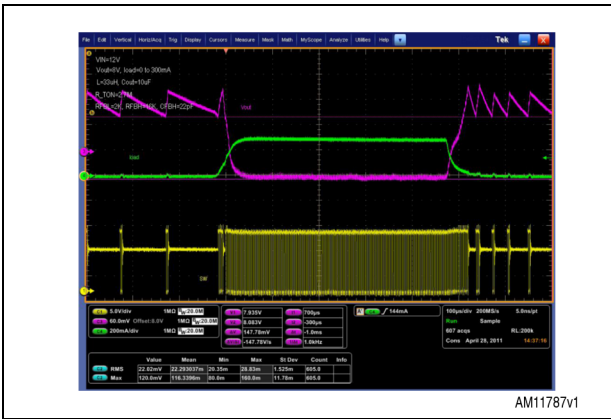
Figure 28. Load step = 0 to 300 mA
