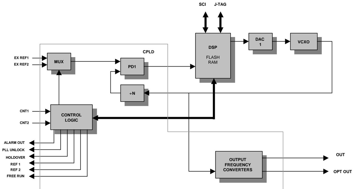
Figure 1. - The functional block diagram of SY0006
