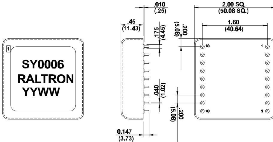
Figure 5 – The mechanical dimensions.
