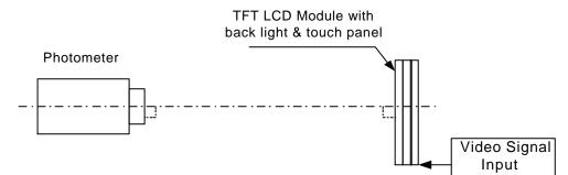
Note 9-1: Viewing angle diagrams (Measure System B)
