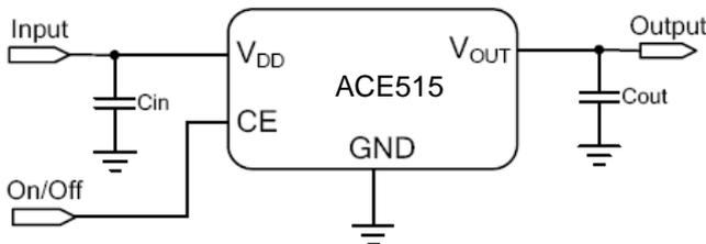
Note Input capacitor (C<sub>in</sub>=1uF) and Output capacitor (C<sub>out</sub>=1uF) are recommended in all application circuit.
