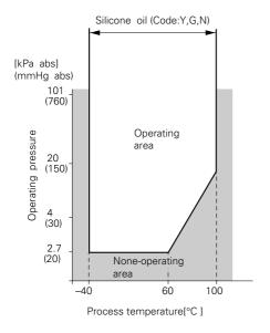
Fig. 1 Relation between process temperature and operating pressure
