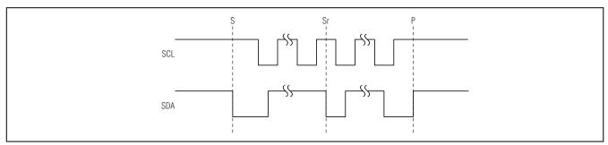
Figure 7. START, STOP, and REPEATED START Conditions
