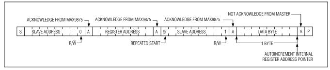
Figure 11. Reading One Indexed Byte of Data from the MAX9875
