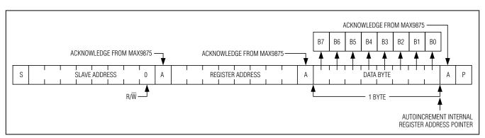
Figure 9. Writing One Byte of Data to the MAX9875
