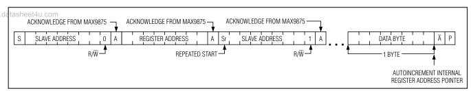
Figure 12. Reading n-Bytes of Indexed Data from the MAX9875
