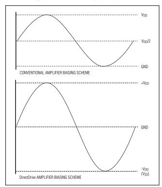
Figure 5. Traditional Amplifier Output vs. MAX9875 DirectDrive Output
