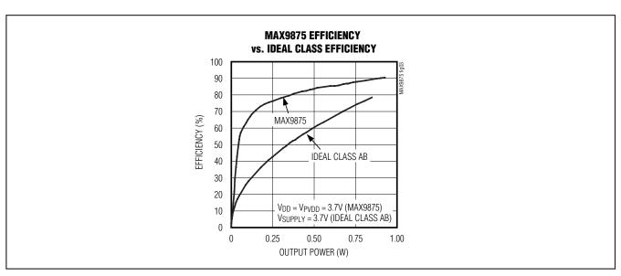
Figure 3. MAX9875 Efficiency vs. Class AB Efficiency
