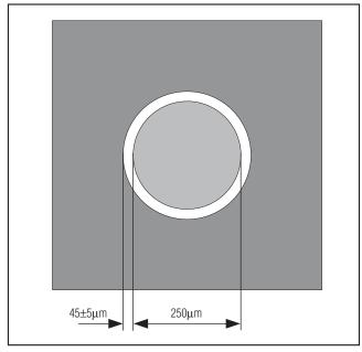
Figure 15. PCB Footprint Recommendation Diagram
