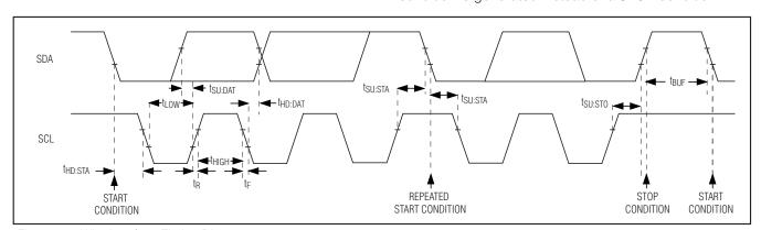
Figure 6. 2-Wire Interface Timing Diagram
