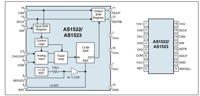
Figure 1. Block Diagram and Pin Assignments
