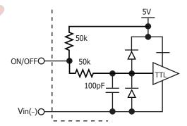
Figure B: Internal ON/OFF pin circuitry
