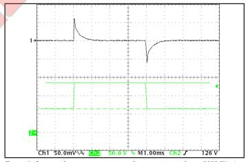
Figure 6: Output voltage response to step-change in input voltage (1000 V/ms). Load cap: 1  $\mu$ F ceramic and 15  $\mu$ F tantalum capacitors. Ch 1: Vout, Ch 2: Vin.
