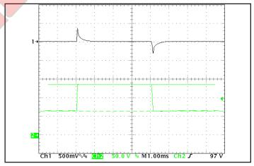
Figure 6: Output voltage response to step-change in input voltage (1000 V/ms). Load cap: 1 µF ceramic and 15 µF tantalum capacitors. Ch 1: Vout, Ch 2: Vin.
