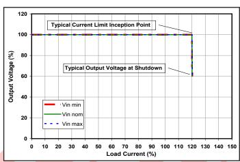
Common Figure 2: Output voltage vs. load current showing typical current limit Common Figure 2: Output voltage vs. load current showing typical current limit curves and converter shutdown points.
