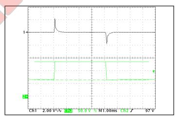
Figure 6: Output voltage response to step-change in input voltage (1000 V/ms). Load cap: 1 µF ceramic capacitor. Ch 1: Vout, Ch 2: Vin.
