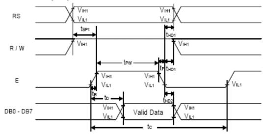
(2) Read mode timing diagram (Read Data from SPLC780C to MPU)
