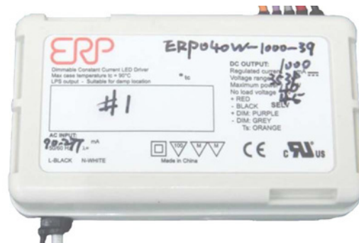
Figure 4: CXA2530 retail track light driver
