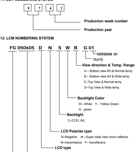
A –TFT analog D –TFT digital Series code 050605–, 5.6 inch Model type
