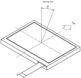
Note 8. Measured at the center area of the panel when all the input terminals of LCD panel are electrically opened.
