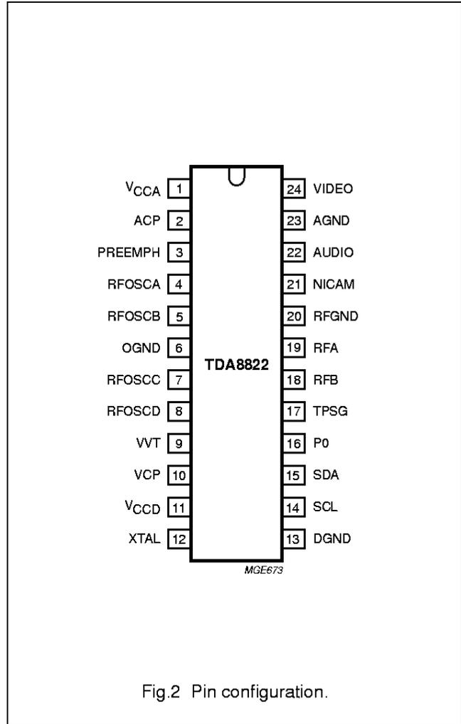
Fig.2 Pin configuration.
