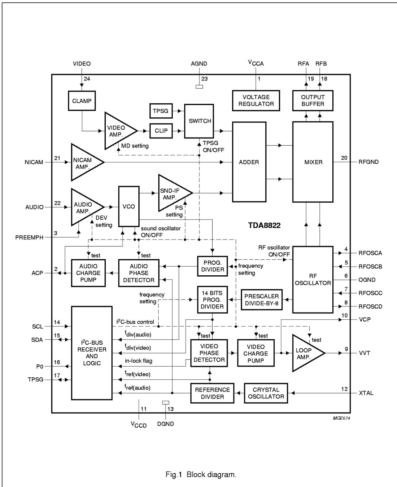
Fig.1 Block diagram.
