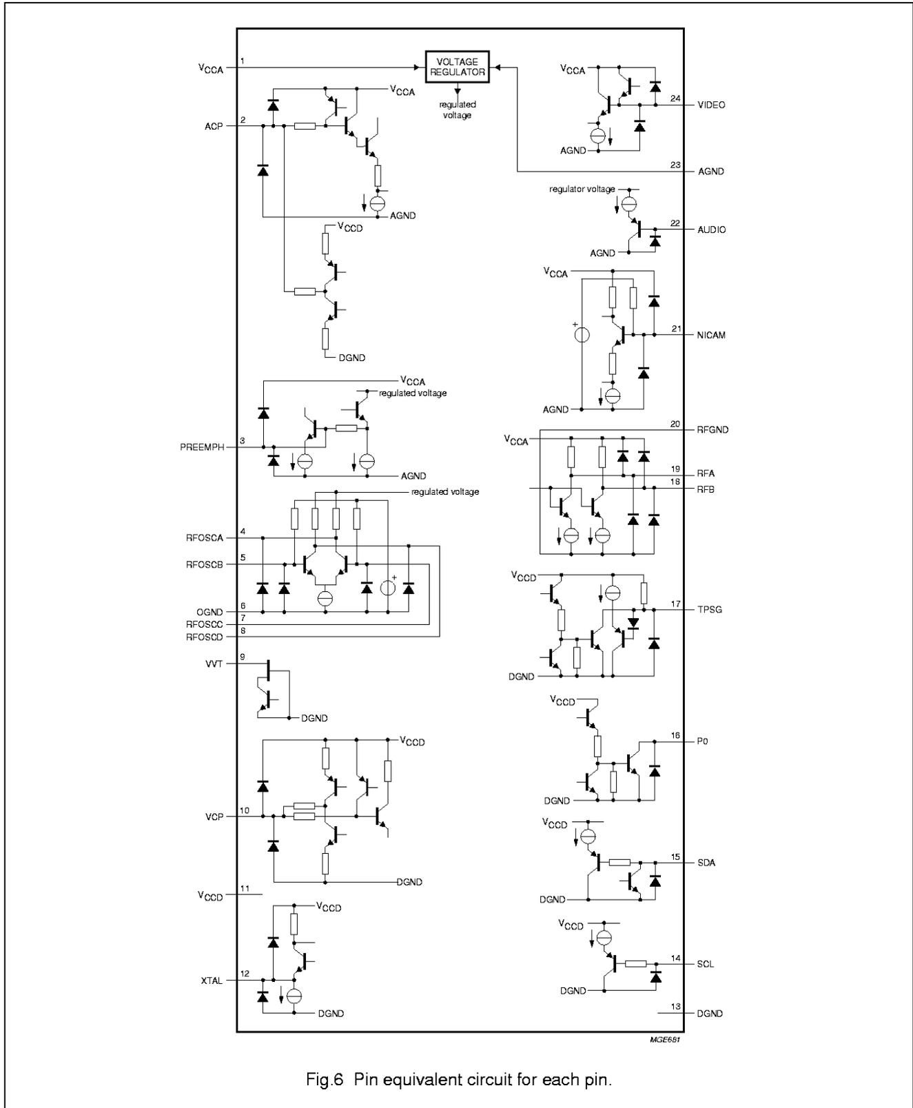
Fig.6 Pin equivalent circuit for each pin.
