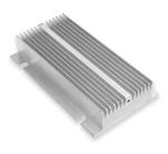
The CFH is a high quality range of aluminium housed power resistors offering environmental protection to IP55, 6kV dielectric strength, 1.8kW power dissipation, and the ability to absorb electrical pulses of up to 24kJ.
