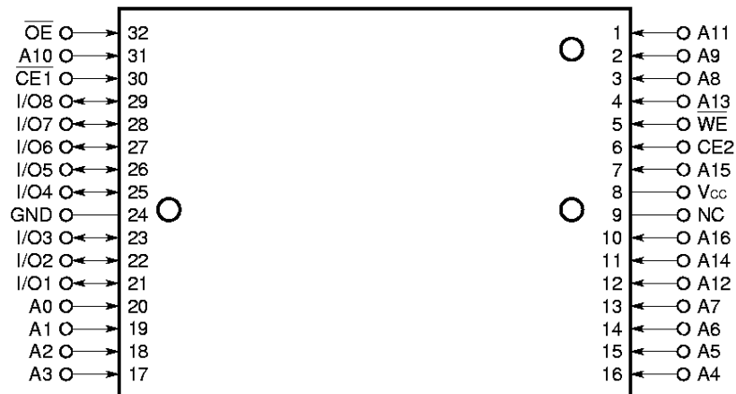
32-pin Plastic TSOP (I) (8 × 13.4mm) (Reverse bent) [ \mu PD431000AGU-9KH]
