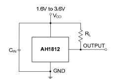
Note: 4.  $C_{IN}$  is for power stabilization and to strengthen the noise immunity, the recommended capacitance is 10nF to 100nF. R<sub>L</sub> is the pull-up resistor, the recommended resistance is 10k\Omega to 100kΩ.
