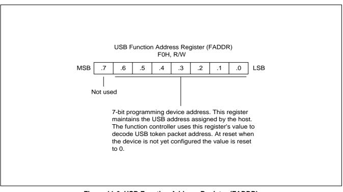
Figure 11-6. USB Function Address Register (FADDR)
