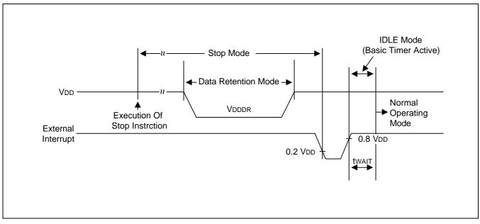
Figure 15-3. Stop Mode Release Timing When Initiated by an External Interrupt
