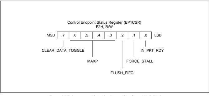
Figure 11-8. Interrupt Endpoint Status Register (EP1CSR)
