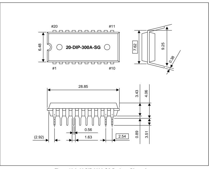
Figure 16-2. 20-DIP-300A-SG Package Dimensions
