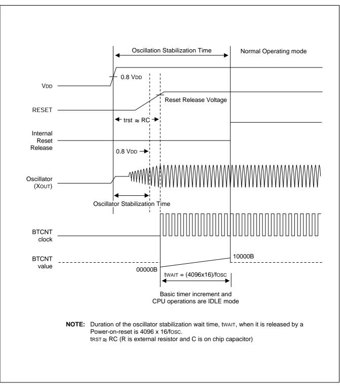
Figure 10-2. Oscillation Stabilization Time on RESET Pin Used
