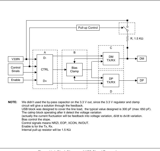
Figure 11-4. Block Diagram of USB Signal Transceiver
