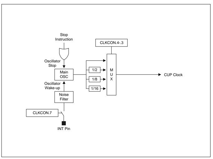
Figure 7-5. System Clock Circuit Diagram
