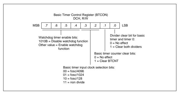
Figure 10-1. Basic Timer Control Register (BTCON)
