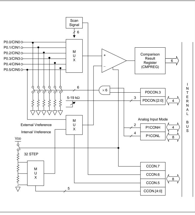
Figure 12-3. Comparator Functional Block Diagram
