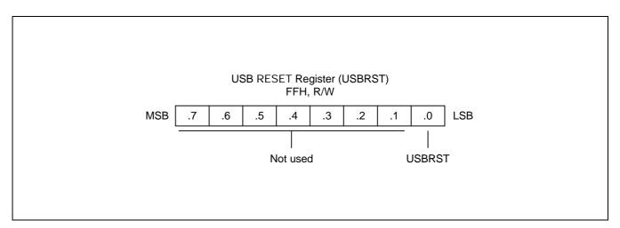
Figure 11-12. USB RESET Register (USBRST)
