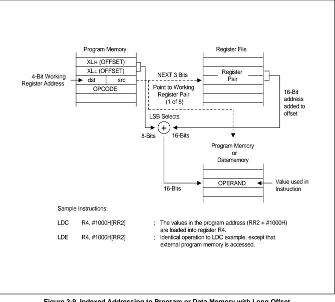
Figure 3-9. Indexed Addressing to Program or Data Memory with Long Offset
