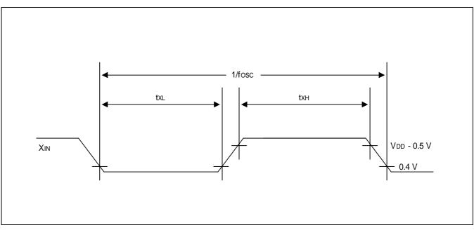
Figure 15-2. Clock Timing Measurement Points at X<sub>IN</sub>
