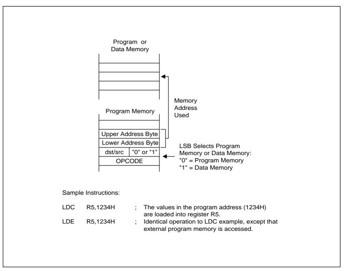
Figure 3-10. Direct Addressing for Load Instructions
