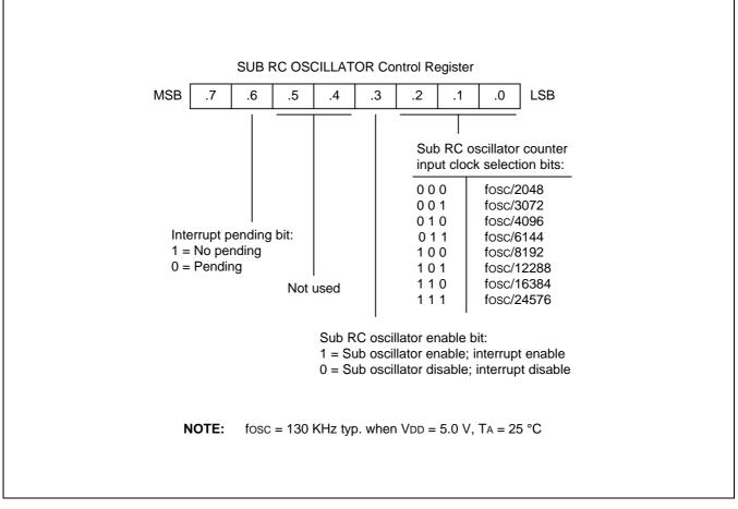
Figure 13-1. SUB RC OSCILLATOR Control Register
