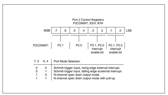
Figure 9-5. Port Control Registers (P2CONINT)
