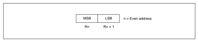
Figure 2-3. 16-Bit Register Pairs
