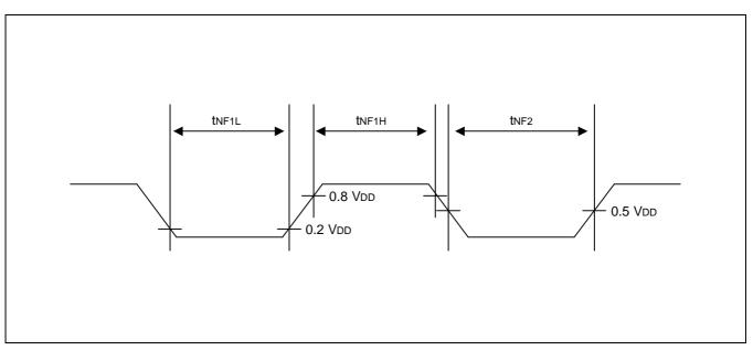
Figure 15-1. Nose Filter Timing Measurement Points
