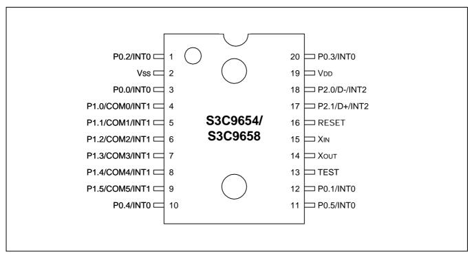
Figure 1-2. Pin Assignment (20 Pin)
