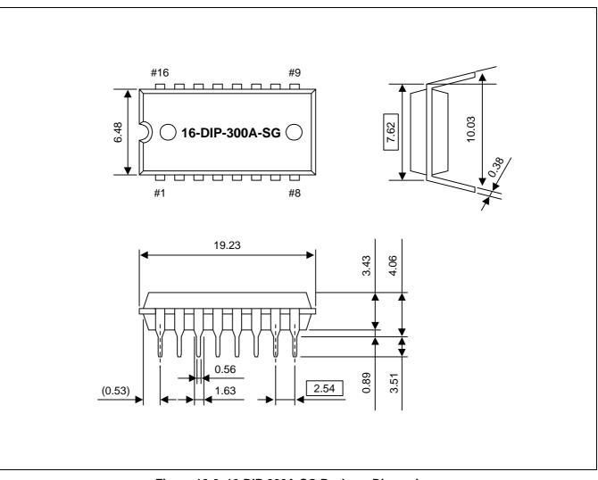
Figure 16-6. 16-DIP-300A-SG Package Dimensions
