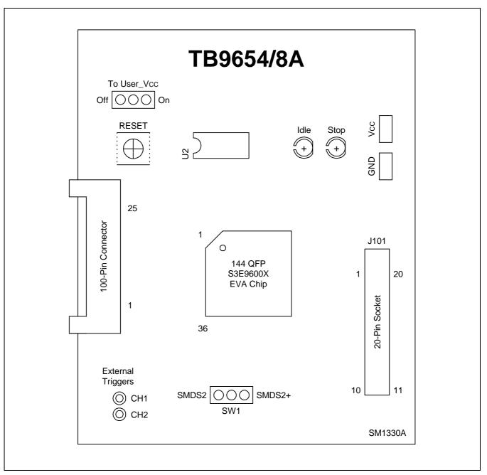
Figure 18-2. TB9654/8A Target Board Configuration
