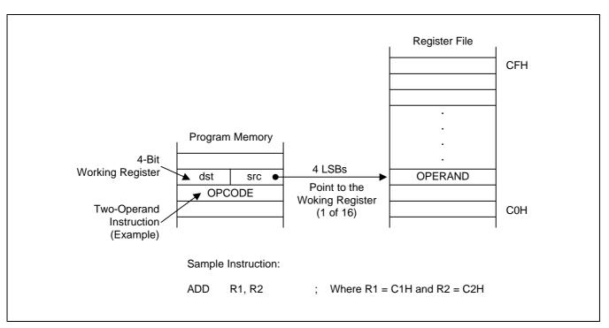
Figure 3-2. Working Register Addressing
