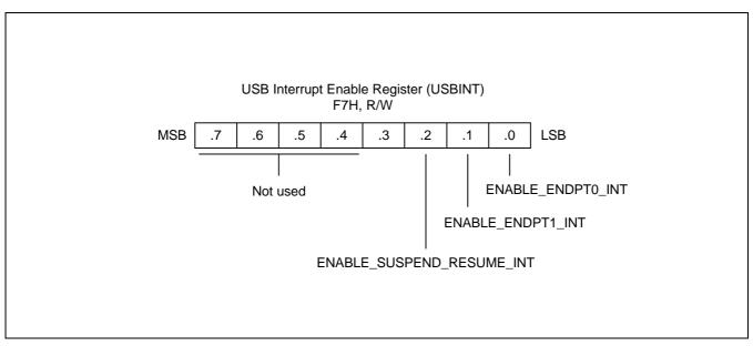
Figure 11-10. USB Interrupt Enable Register (USBINT)
