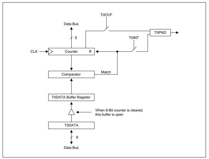
Figure 10-5. Simplified Timer 0 Function Diagram: Interval Timer Mode
