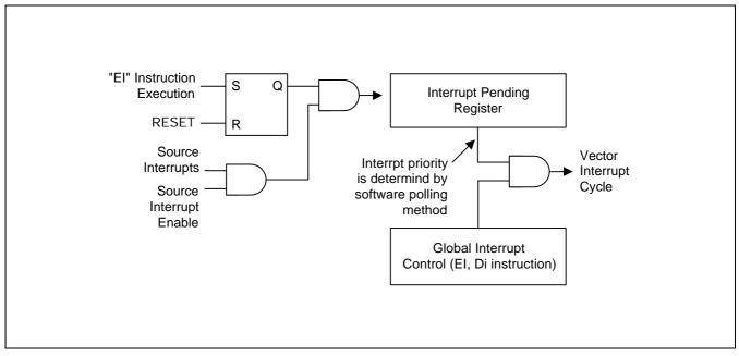
Figure 5-2. Interrupt Function Diagram
