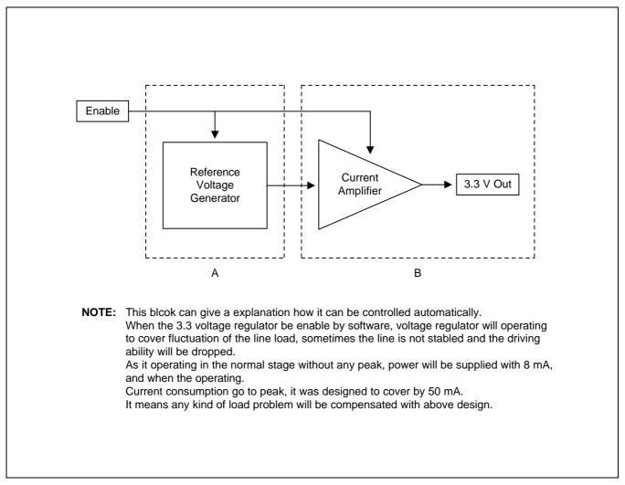
Figure 11-3. Block Diagram of Voltage Regulator
