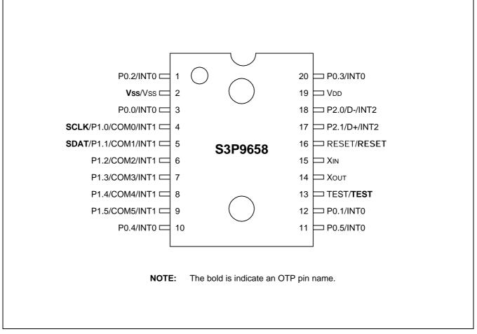
Figure 17-1. S3P9658 Pin Assignments (20 Pin)
