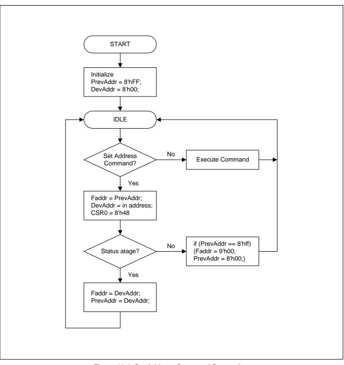
Figure 19-1. Set Address Command Supporting
