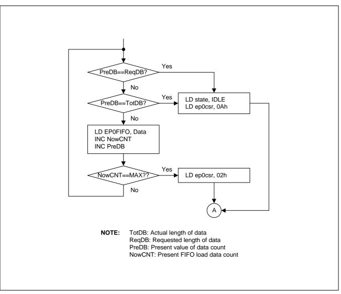
Figure 19-4. EP0FIFO Loading Part
