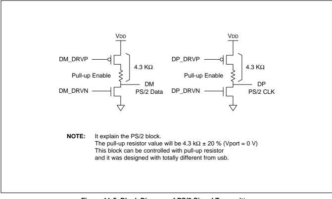
Figure 11-5. Block Diagram of PS/2 Signal Transmitter
