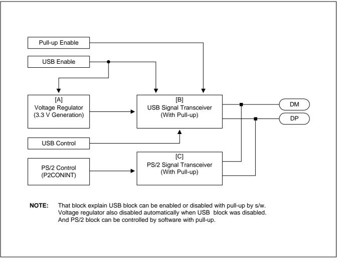
Figure 11-2. Block Diagram of USB and PS/2 Transceiver
