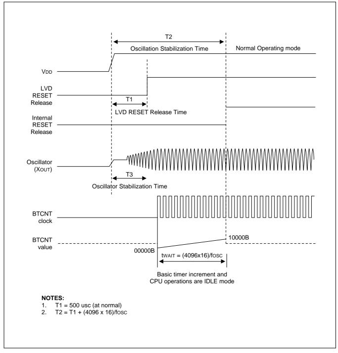
Figure 14-3. LVR and Power On RESET Operation
