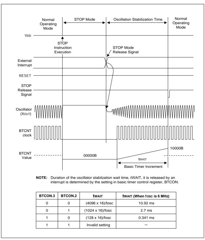
Figure 10-3. Oscillation Stabilization Time on STOP Mode Release
