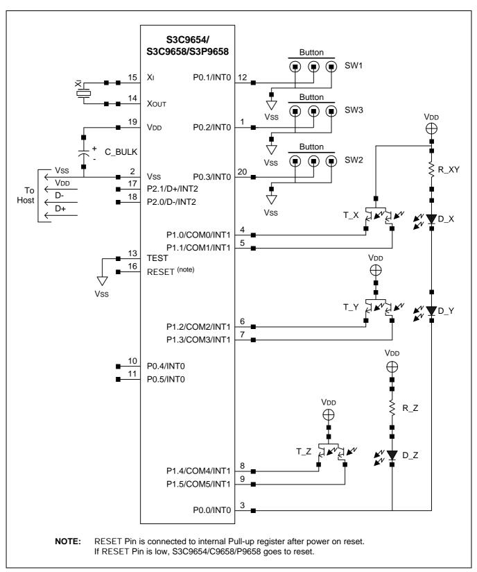
Figure 1-9. USB Mouse Circuit Diagram
