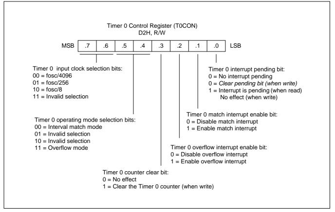
Figure 10-4. Timer 0 Control Register (T0CON)
