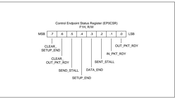
Figure 11-7. Control Endpoint Status Register (EP0CSR)
