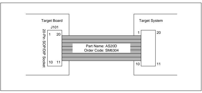
Figure 18-4. TB9654/8A Adapter Cable for 20-SOP/DIP Package
