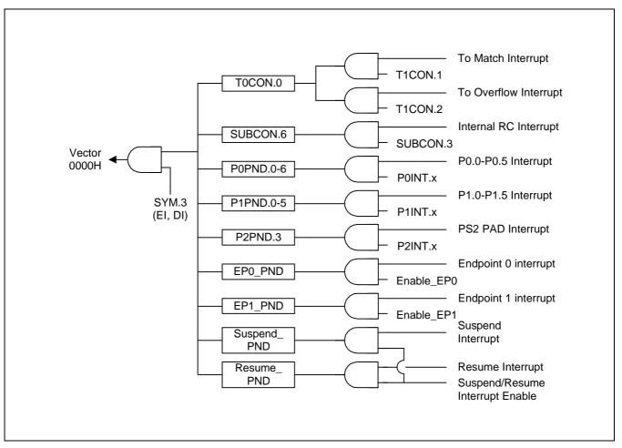
Figure 5-3. S3C9654/C9658/P9658 Interrupt Structure
