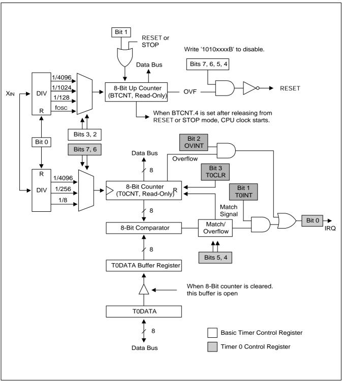
Figure 10-6. Basic Timer and Timer 0 Block Diagram
