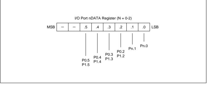
Figure 9-1. Port Data Register Format
