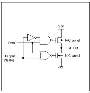
Figure 1-5. Pin Circuit Type C
