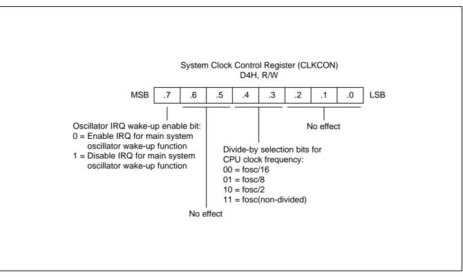
Figure 7-4. System Clock Control Register (CLKCON)
