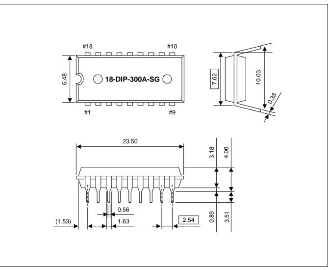
Figure 16-4. 18-DIP-300A-SG Package Dimensions
