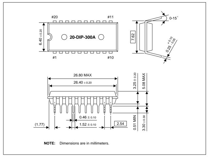
Figure 16-1. 20-DIP 300A Package Dimensions
