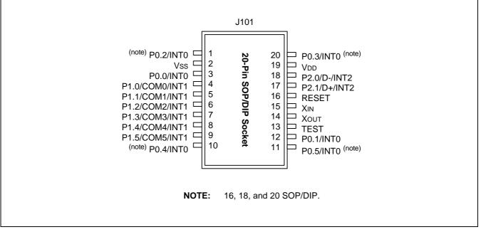
Figure 18-3. 20-Pin Socket for TB9654/8A
