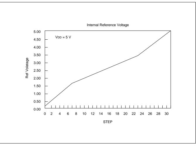
Figure 12-2. Internal Reference Voltage (Hysteresis)
