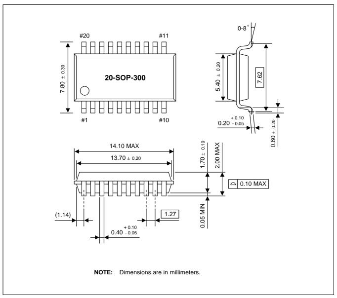
Figure 16-3. 20-SOP-300 Package Dimensions
