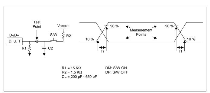
Figure 15-4. USB Data Signal Rise and Fall Time
