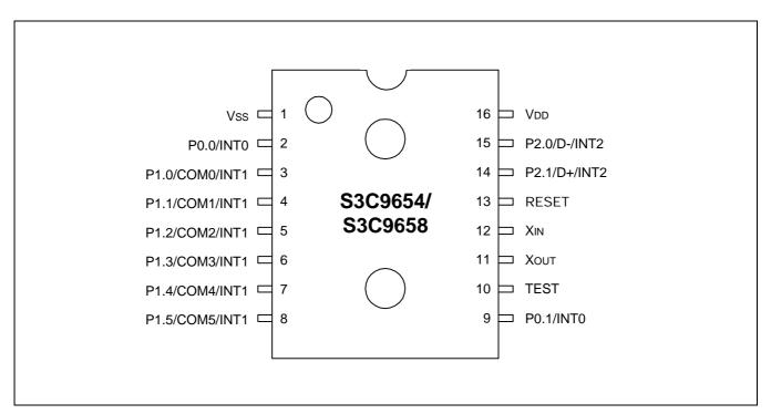
Figure 1-4. Pin Assignment (16 Pin)
