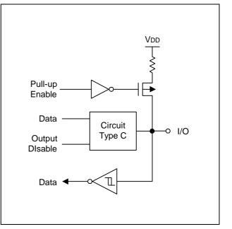
Figure 1-6. Pin Circuit Type D
