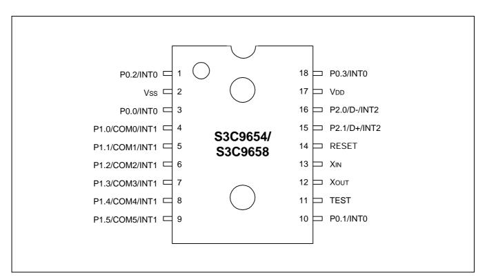
Figure 1-3. Pin Assignment (18 Pin)
