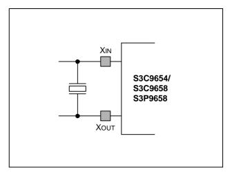
Figure 7-2. Main Oscillator Circuit (Crystal/Ceramic Oscillator)
