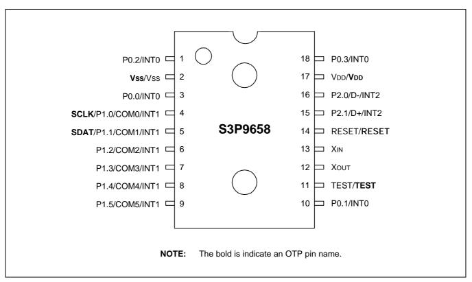
Figure 17-2. S3P9658 Pin Assignments (18 Pin)
