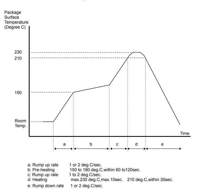
Reflow Soldering process recommendation profile
