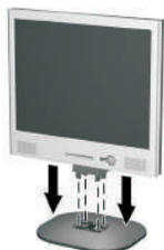
Inserting the Monitor into the Pedestal Base
