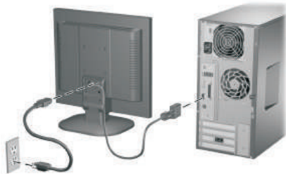
Connecting the VGA and Power Cables
