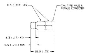
NOTE: All dimensions are given in mm (inches) and are maximum, unless otherwise specified.
