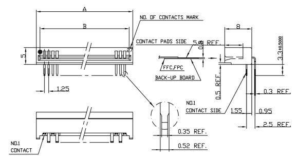
MATERIAL: INSULATOR : PBT RESIN GLASS REINFORCED (UL94V-0)
