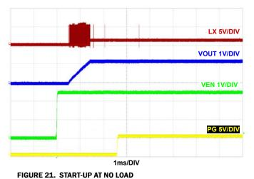
F<sub>SW</sub> = 2MHz, V<sub>IN</sub> = 5V, MODE = PFM, T<sub>A</sub> = +25°C
