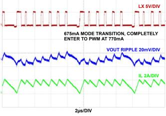
FIGURE 49. PFM TO PWM TRANSITION  $F_{SW}$  = 2MHz,  $V_{IN}$  = 5V, MODE = PFM,  $T_A$  = +25 °C
