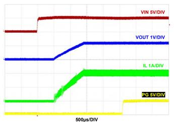
FIGURE 33. START-UP V<sub>IN</sub> AT 2A LOAD  $F_{SW} = 2MHz$ , V<sub>IN</sub> = 5V, MODE = PFM, T<sub>A</sub> = +25°C
