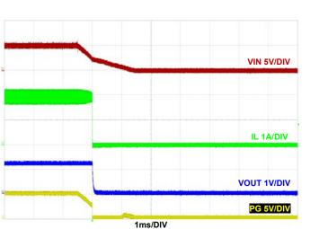
FIGURE 35. SHUTDOWN V<sub>IN</sub> AT 2A LOAD  $F_{SW} = 2MHz$ , V<sub>IN</sub> = 5V, MODE = PFM, T<sub>A</sub> = +25°C
