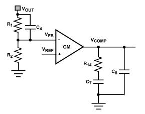
FIGURE 56. TYPE II COMPENSATOR
