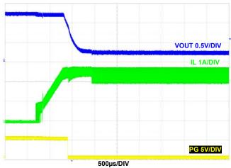
FIGURE 48. OVERCURRENT PROTECTION  $F_{SW} = 2MHz$ ,  $V_{IN} = 5V$ , MODE = PWM,  $T_A = +25$  °C
