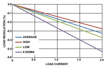
FIGURE 14. LOAD REGULATION,  $T_A = +105^\circ$ , 5.5V<sub>IN</sub>, 0.6V<sub>OUT</sub>, 1MHz
