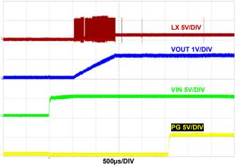
FIGURE 37. START-UP V<sub>IN</sub> AT NO LOAD  $F_{SW} = 2MHz$ , V<sub>IN</sub> = 5V, MODE = PFM, T<sub>A</sub> = +25°C
