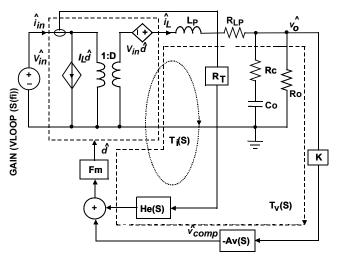
FIGURE 55. SMALL SIGNAL MODEL OF SYNCHRONOUS BUCK REGULATOR
