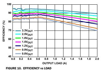
$F_{SW} = 1MHz$ ,  $V_{IN} = 5V$ , MODE = PFM,  $T_A = +25$  °C
