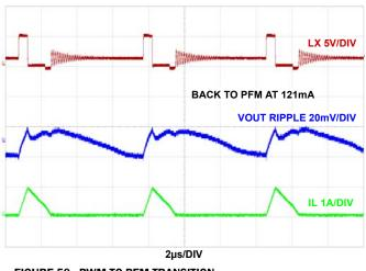
FIGURE 50. PWM TO PFM TRANSITION  $F_{SW} = 2MHz$ ,  $V_{IN} = 5V$ , MODE = PWM,  $T_A = +25$  °C
