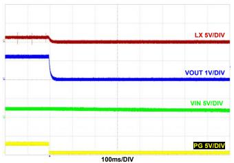
FIGURE 39. SHUTDOWN V<sub>IN</sub> AT NO LOAD  $F_{SW} = 2MHz$ , V<sub>IN</sub> = 5V, MODE = PFM, T<sub>A</sub> = +25°C
