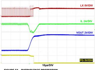
FIGURE 51. OVERVOLTAGE PROTECTION  $F_{SW} = 2MHz$ ,  $V_{IN} = 5V$ , MODE = PFM,  $T_A = +25$  °C
