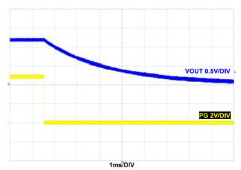
FIGURE 52. OVER-TEMPERATURE PROTECTION  $F_{SW}$  = 2MHz, V<sub>IN</sub> = 5V, MODE = PWM, T<sub>A</sub> = +163 °C
