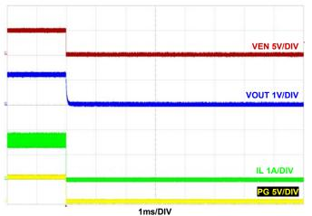
FIGURE 30. SHUTDOWN AT 1.5A LOAD  $F_{SW} = 2MHz$ ,  $V_{IN} = 5V$ , MODE = PWM,  $T_A = +25$  °C
