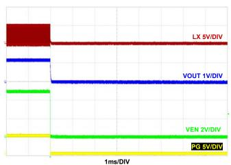
FIGURE 26. SHUTDOWN AT 2A LOAD F<sub>SW</sub> = 2MHz, V<sub>IN</sub> = 5V, MODE = PWM, T<sub>A</sub> = +25°C
