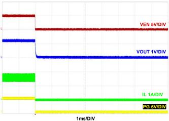
FIGURE 32. SHUTDOWN AT 1.5A LOAD  $F_{SW} = 2MHz$ ,  $V_{IN} = 5V$ , MODE = PFM,  $T_A = +25$ °C
