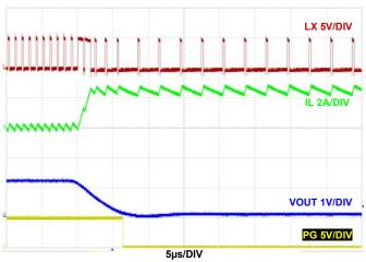
FIGURE 47. OUTPUT SHORT-CIRCUIT  $F_{SW} = 2MHz$ ,  $V_{IN} = 5V$ , MODE = PFM,  $T_A = +25$  °C
