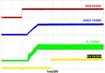
FIGURE 29. START-UP AT 1.5A LOAD  $F_{SW}$  = 2MHz, V<sub>IN</sub> = 5V, MODE = PWM, T<sub>A</sub> = +25°C
