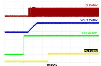
FIGURE 22. START-UP AT NO LOAD F<sub>SW</sub> = 2MHz, V<sub>IN</sub> = 5V, MODE = PWM, T<sub>A</sub> = +25°C
