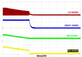
FIGURE 40. SHUTDOWN V<sub>IN</sub> AT NO LOAD  $F_{SW} = 2MHz$ , V<sub>IN</sub> = 5V, MODE = PWM, T<sub>A</sub> = +25°C
