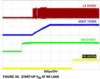
$F_{SW} = 2MHz$ ,  $V_{IN} = 5V$ , MODE = PFM,  $T_A = +25^{\circ}C$
