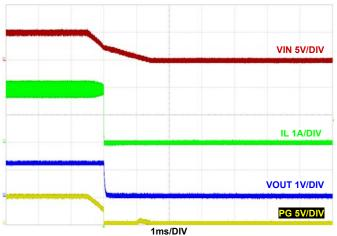
FIGURE 36. SHUTDOWN V<sub>IN</sub> AT 2A LOAD  $F_{SW}$  = 2MHz, V<sub>IN</sub> = 5V, MODE = PWM, T<sub>A</sub> = +25 °C
