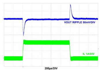
FIGURE 46. LOAD TRANSIENT  $F_{SW} = 2MHz$ ,  $V_{IN} = 5V$ , MODE = PWM,  $T_A = +25^{\circ}C$
