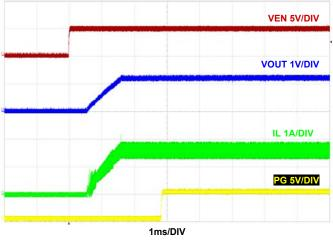
FIGURE 31. START-UP AT 1.5A LOAD  $F_{SW}$  = 2MHz,  $V_{IN}$  = 5V, MODE = PFM,  $T_A$  = +25 °C
