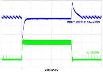
FIGURE 45. LOAD TRANSIENT  $F_{SW}$  = 2MHz,  $V_{IN}$  = 5V, MODE = PFM,  $T_A$  = +25°C
