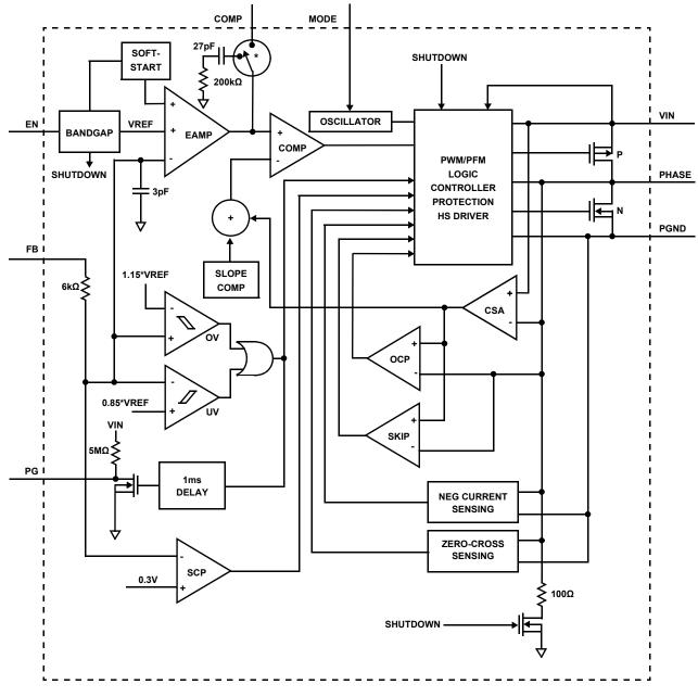
\* By default, when COMP is tied to VIN, the voltage loop is internally compensated with the 27pF and 200kΩ RC network. Please see "COMP" pin in the "Pin Descriptions" table on page 4 for more details.
