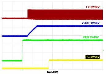
FIGURE 27. START-UP AT 2A LOAD  $F_{SW} = 2MHz$ ,  $V_{IN} = 5V$ , MODE = PFM,  $T_A = +25$  °C
