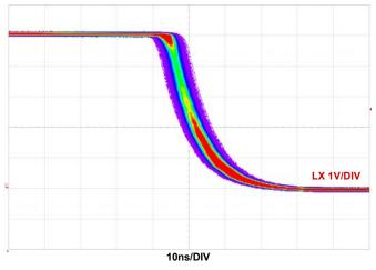
FIGURE 41. JITTER AT NO LOAD  $F_{SW} = 2MHz$ ,  $V_{IN} = 5V$ , MODE = PWM,  $T_A = +25$  °C
