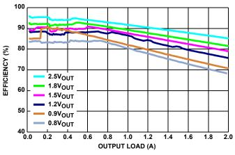
FIGURE 6. EFFICIENCY vs LOAD  $F_{SW}$  = 1MHz,  $V_{IN}$  = 3.3V, MODE = PFM,  $T_A$  = +25 °C
