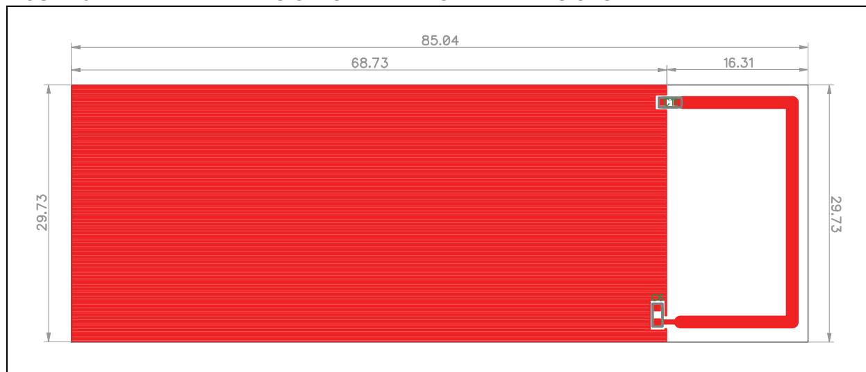
FIGURE 3: ANTENNA DESIGN. OVERALL BOARD DIMENSIONS
