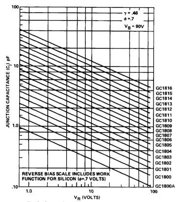
**Typical Junction Capacitance vs Reverse Bias**
