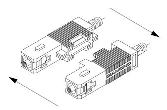
DIAMOND also offers a hybrid mating adaptor which permits mating of SC Duplex plugs to ST™-style connectors.
