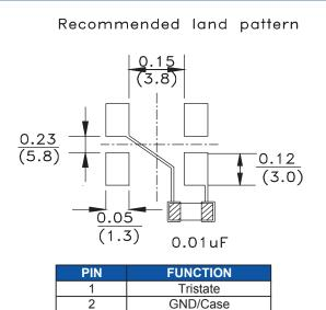
Note: Recommend using an approximately 0.01uF bypass capacitor between pin 2 and 4.
