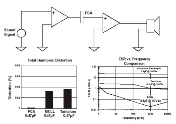
Using FCA capacitors in audio circuits can result in lower sound distortion. The low e.s.r., the absence of piezoelectric effects, and the non polar nature of the capacitor will eliminate sources of distortion in your audio circuits.
