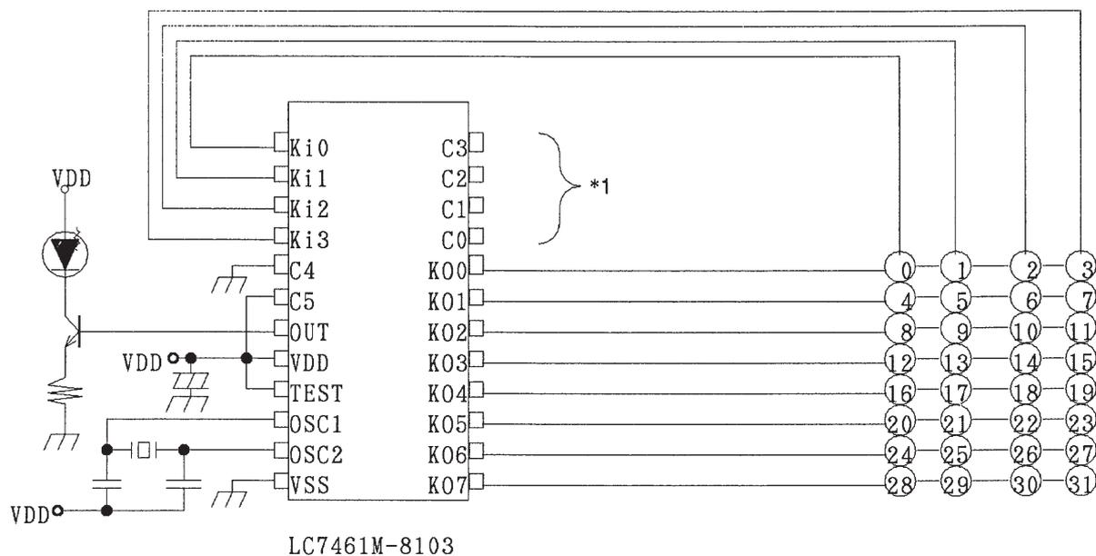
Note: \*1. The states of C0 to C3 should be set to match the diode matrix. (0 = GND, 1 = V<sub>DD</sub>)
