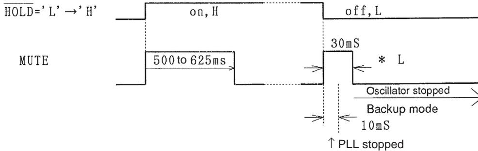
\* Since the MUTE pin goes to the high impedance state, a pull down resistor is used to hold it at the low level.
