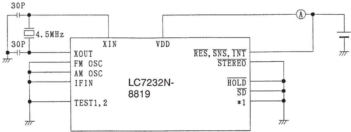
Notes: T0, T1, T2, T3, T4, T5, T6, T7, POWOUT, MUTE, T-ON, BASS, CLK, CE, VDN, VUP, SW2/A/B, LW/SW1, MW, FM/AM, MO/ST = "Open"
