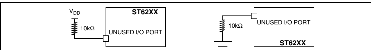
Figure 56. Two typical Applications with unused I/O Pin
