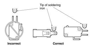
When soldering automatically, adjust the amount of solder so that flux does not float onto the top of PCB. If flux enters the switch, it can cause contact failure.
