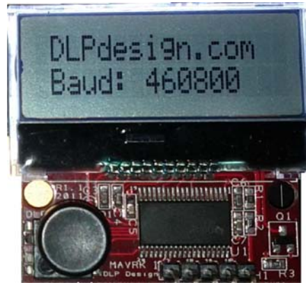
Figure 2: DLP-MAV-LCD1 Module Ready to Start Right Out of the Box
