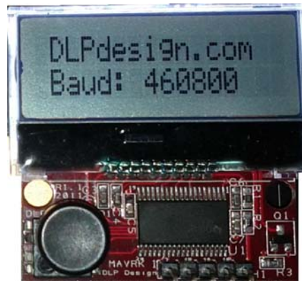
Figure 4: Splash Screen on Power Up
