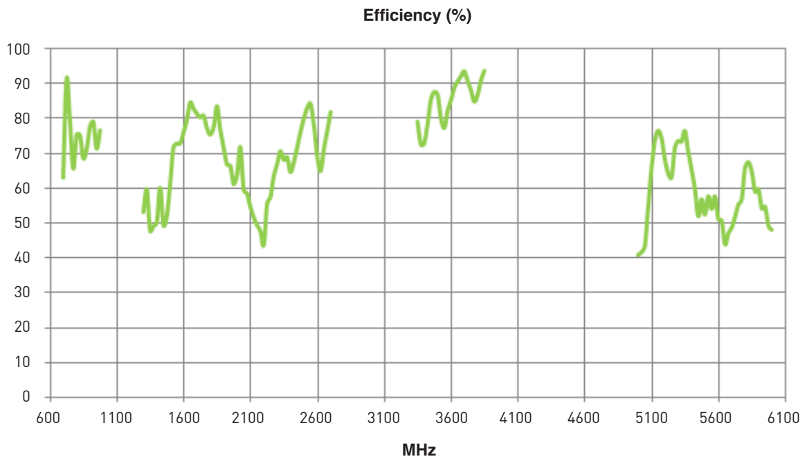
Figure 4. Efficiency of FXUB66 UWB Antenna.
