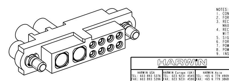
INSERTION FORCE = 5N MAX WITHDRAWAL FORCE = 0.5N MIN
