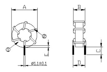
UNIT: mm A=14.0MAX. B=8.0MAX. C=3.5±0.5 D=5.0±0.5 E=0.5MIN
