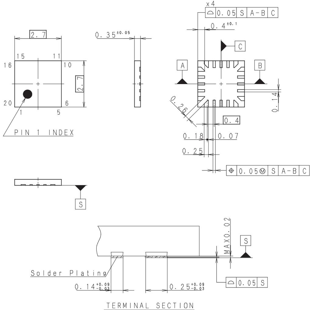
Note:Cutting burr of lead are 0.05mm MAX.
