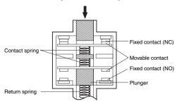
Conforms to EN60947-5-1 Direct Opening Operation ⊕
