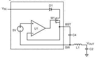
Figure 2—Internal Bootstrap Charging Circuit
