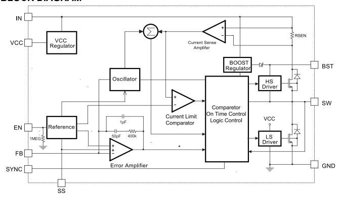
Figure 3—Block Function Diagram
