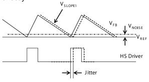
Figure 3—Jitter in PWM Mode
