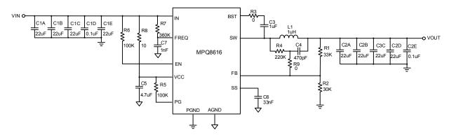
Figure 14 — Typical Application Circuit with Low ESR Ceramic Capacitor MPQ8616, V<sub>IN</sub>=5V, V<sub>OUT</sub>=1.2V, I<sub>OUT</sub>=6/12A, f<sub>SW</sub>=600kHz
