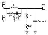
Figure8—Simplified Circuit of Ceramic Capacitor
