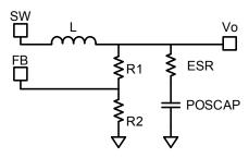
Figure 4—Simplified Circuit in PWM Mode without External Ramp Compensation
