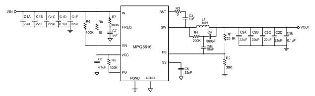
Figure 15 — Typical Application Circuit with Low ESR Ceramic Capacitor and DC-Blocking Capacitor.
