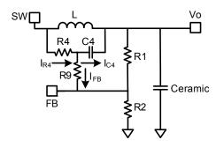
Figure 5—Simplified Circuit in PWM Mode with External Ramp Compensation
