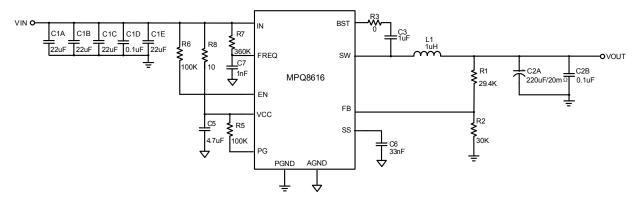
Figure 13 — Typical Application Circuit with No External Ramp MPQ8616, V<sub>IN</sub>=5V, V<sub>OUT</sub>=1.2V, I<sub>OUT</sub>=6/12A, f<sub>SW</sub>=600kHz
