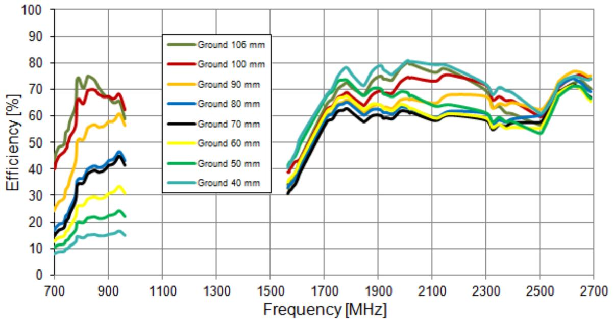
Figure 4. Efficiency of the Warrior PA710 LTE antenna
