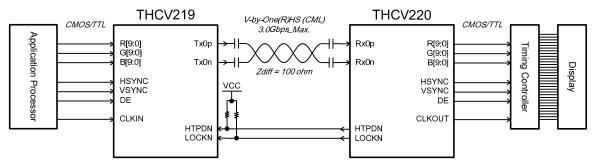
Example for CMOS/TTL to CMOS/TTL
