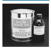
DeltaBond<sup>™</sup> 154 is a medium viscosity, aluminum-filled resin with the best thermal conductivity of this series. It is, however, neither a good electrical insulator nor conductor. Its principal application is that of a good thermal mechanical adhesive for applications such as bonding fins to base plates or structural mounting blocks or brackets to heat sinks. Order one bottle of hardener A4 or B4 per one quart of DeltaBond<sup>™</sup> 154 separately. Shelf life: 3 years.
