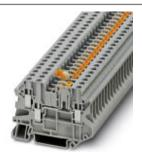
Knife disconnect terminal block, Connection method: Screw connection, Cross section: 0.14 mm² - 6 mm², AWG: 26 - 10, Width: 6.2 mm, Color: gray, Mounting type: NS 35/7,5, NS 35/15
