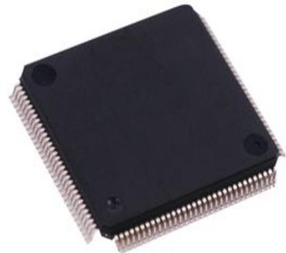
The XRT86VL30 contains an integrated DS1/E1/J1 framer and LIU which provides DS1/E1/J1 framing and error accumulation in accordance with ANSI/ ITU\_T specifications. The framer has its own framing synchronizer and transmit-receive slip buffers. The slip buffers can be independently enabled or disabled as required and can be configured to frame to the common DS1/E1/J1 signal formats.
