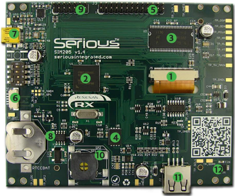
1. 4.3" Wide QVGA 16-bit color 480x272 TFT Touch Display with 4-wire Resistive Touch
