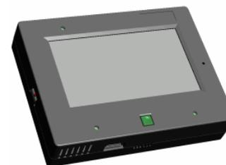
is a prototypers enclosure designed for the SIM205, and includes a USB-rechargeable Lithium Ion battery.
