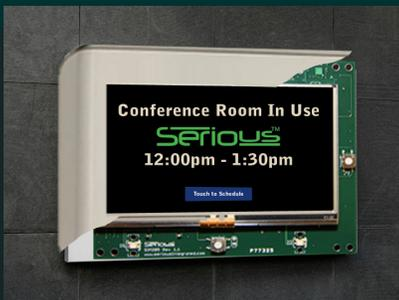
Adding a graphic/touch interface to your product has never been faster than with Serious Integrated Modules. Simply connect power and a communications port from your existing system to the SIM205 and your hardware design is complete.
