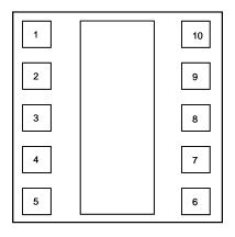
10-Pin Laminate Module Top View (through package)
