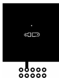
a)  $80^\circ\text{C}/\text{W}$  when mounted on a 1 in<sup>2</sup> pad of 2 oz copper
