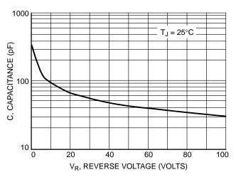
Figure 4. Typical Capacitance
