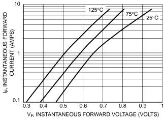
Figure 1. Typical Forward Voltage
