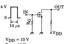
$\begin{array}{l} R_G = 10 \; \Omega \\ D.U. \leq 1\% \\ V_{IN}: \; t_r, \; t_f < 5 \; ns \\ COMMON \; SOURCE \\ Ta = 25^\circ C \end{array}$
